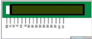
LCD (Liquid Crystal Display) screen is an electronic display module and find a wide range of applications. A 16x2 LCD display is very basic module and is very commonly used in various devices and circuits. These modules are preferred over seven segments and other multi segment LEDs. The reasons being: LCDs are economical; easily programmable; have no limitation of displaying special & even custom characters (unlike in seven segments). Animations and so on.
