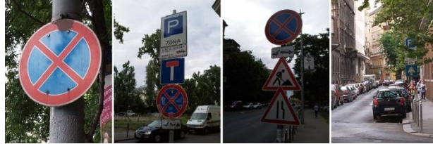
Fig. 1. Example images for ageing, vandalism, occlusion, and an occlusion with rotation, respectively, showing different lighting conditions
