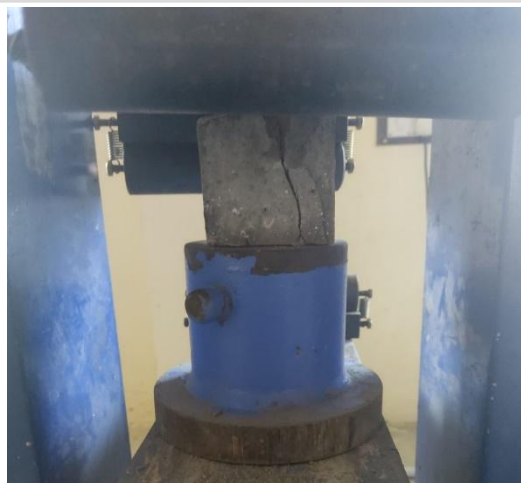
Compressive strength test
