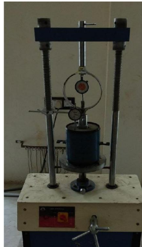
Fig 1: shows the typical test arrangement of the stone column
