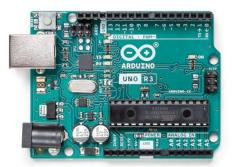
Arduino UNO is a low-cost, flexible, and easy-to-use programmable open-source microcontroller board that can be integrated into a variety of electronic projects.
