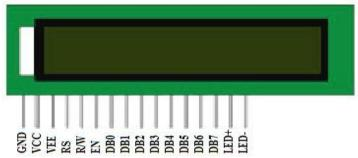
The Figure shows the pin diagram of 16X2 LCD display. In this LCD each character is displayed in 5X7 pixel matrix. While Vcc and GND(Vss) are connected to +5V and ground respectively, Vcc is used for controlling contrast. In this project LCD is used to display message for temperature, humidity, CO2 level, LDR value Light ON/OFF.
