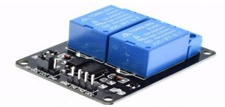
Relay is an electrically operated switch. Many relays use an electromagnet to operate a switching mechanism mechanically. In this project HEJQC3FC relay with maximum current and voltage rating of 7.5A,14V is used, to supply +5V to multi charger connector when it receives enable signal from microcontroller.
