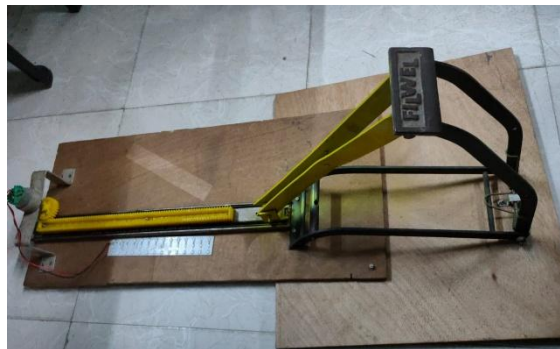
Fig. 3.1 Basic model of Rack and pinion mechanism.
