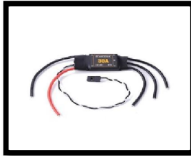
Fig. 7. Electronic speed controller (30A)
