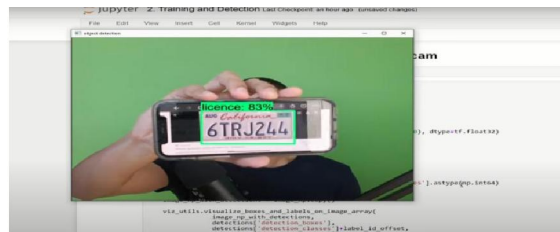
Fig 3. Detection of license plate in real time
