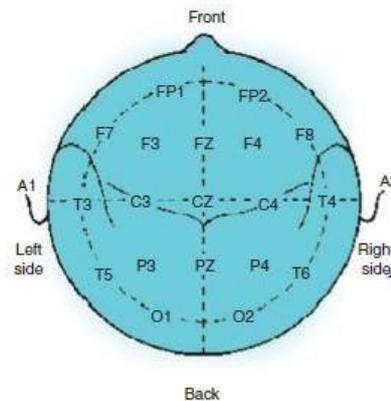
Figure 1 Locations of the EEG electrodes in the international 10–20 system. Used with expressed permission of Brain Master Technologies, Inc.
