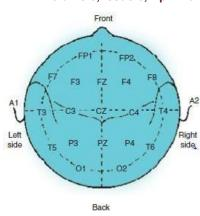
Figure 1 Locations of the EEG electrodes in the international 10–20 system. Used with expressed permission of Brain Master Technologies, Inc.
