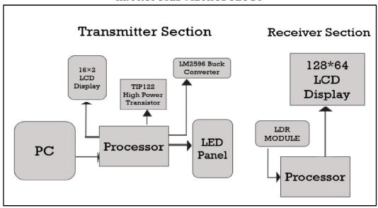
This block diagram describes the working of project 'Image & Text Transmission Using Li-Fi Technology'
