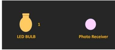
Similarly, when the light source is ON, or we can say that if the current is maximum flowing through the LED, then the illumination of the LED will be maximum. And it will be treated as a digital 1 which will be transmitted at the receiver side.
