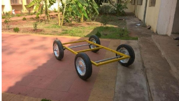
Fig 5.1.8 Frame and shafts with tyres
