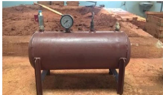
Fig 8 Air Storage tank
