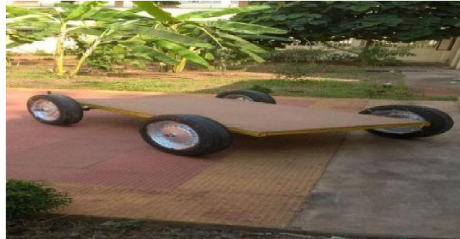
Fig 5.3.2 Frame with wooden plank
