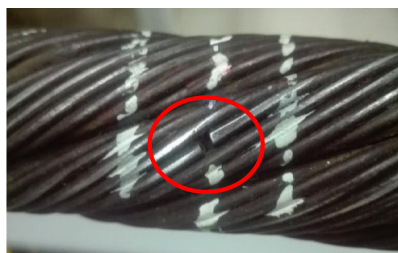
(b) Specimen of outer single broken wire defect in the experiments
