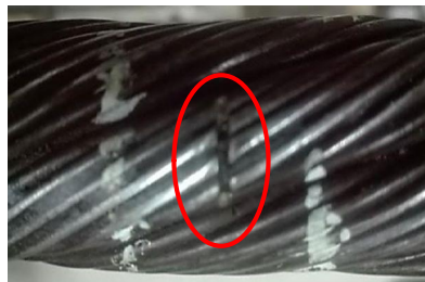
(a) Specimen of outer multiple broken wires defect in the experiments
