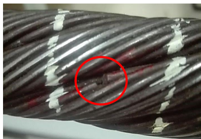
(c) Specimen of inner single broken wire defect in the experiments
