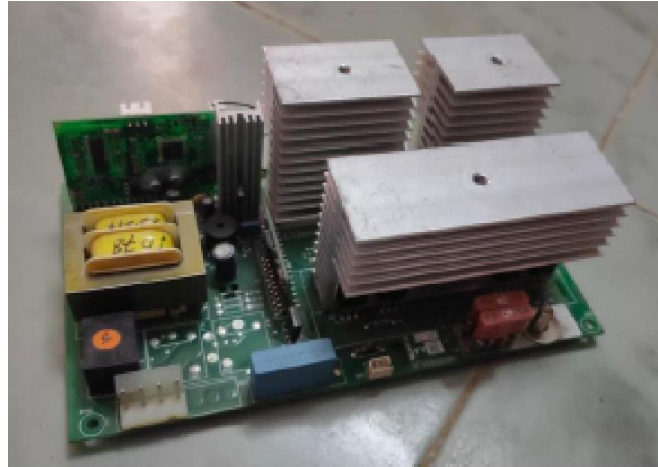
Fig. 4. Inverter Circuit design
