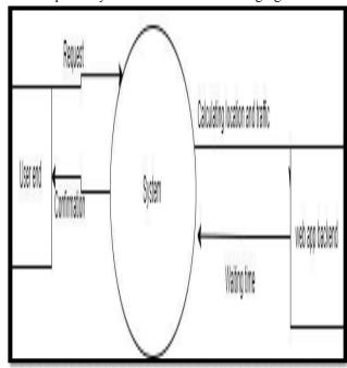
The above diagram features how the data is transferred from one end to the other i.e. the flow of data and control, here firstly the user will enter his credentials, then this data will be transferred to the frontend for primary credentials after verification this data would be sent to backend or server and the necessary computations would be done and the user would be placed into the queue for the charging station
