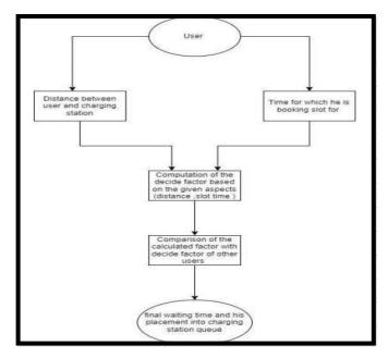
The above diagram shows the implementation of RAWT algorithm, which utilizes the user's distance from charging station, the slot timing and the duration required by the user to reach the charging station
