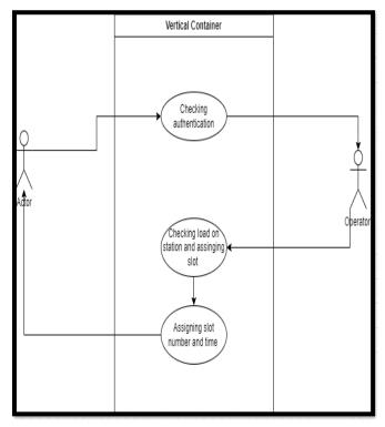
The above use case diagram describes the working of the system with respect to the user's interaction with the system, here the user will make a request for slot booking and accordingly he will be placed into the queue of the charging station
