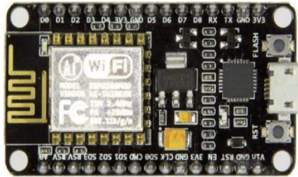
Fig 5 : ESP-12E Based Node MCU
