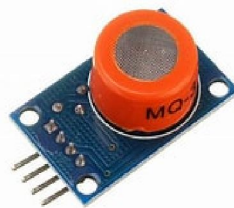
Fig 6 : MQ3 Alcohol Sensor
