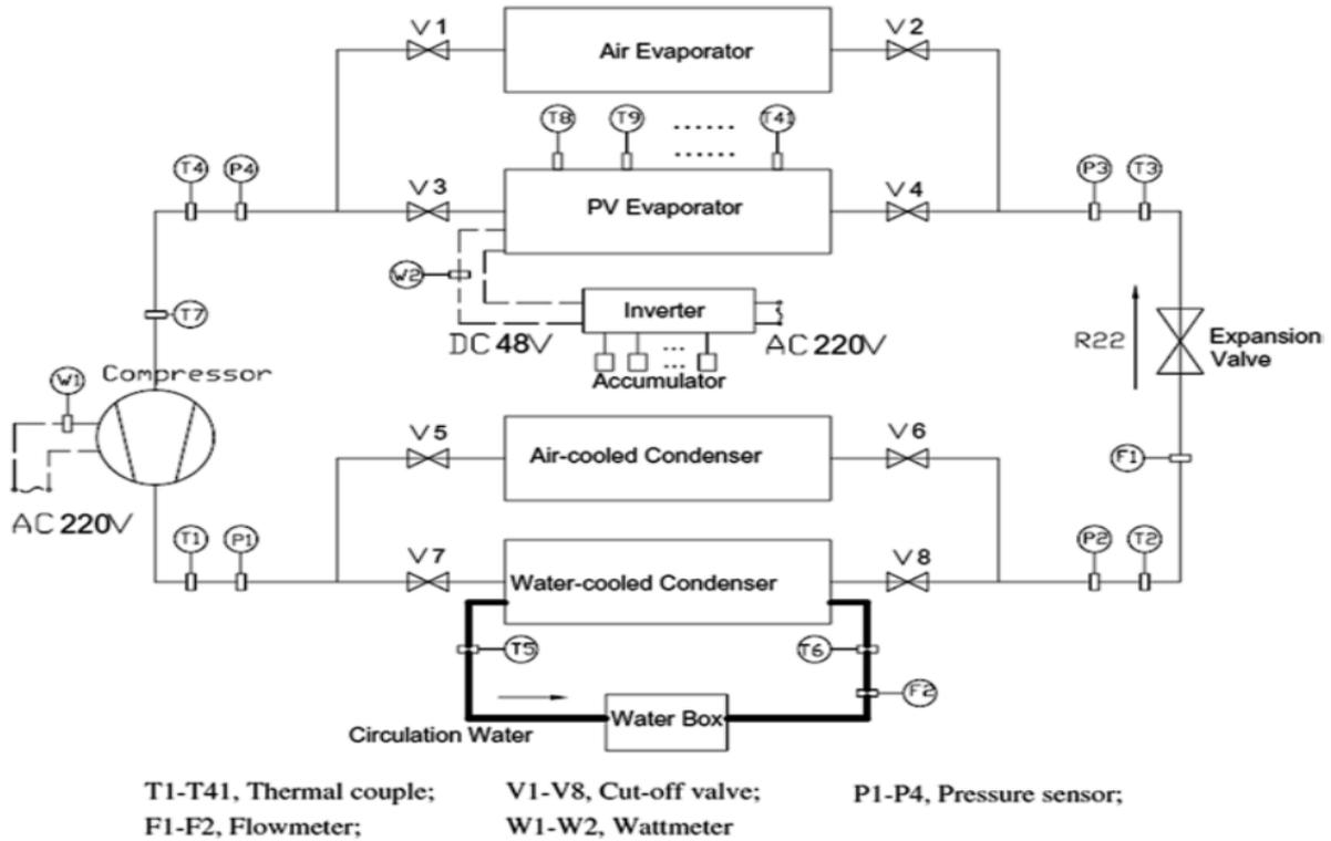
Fig. 5 Schematic diagram of the PV-SAHP experimental setup
