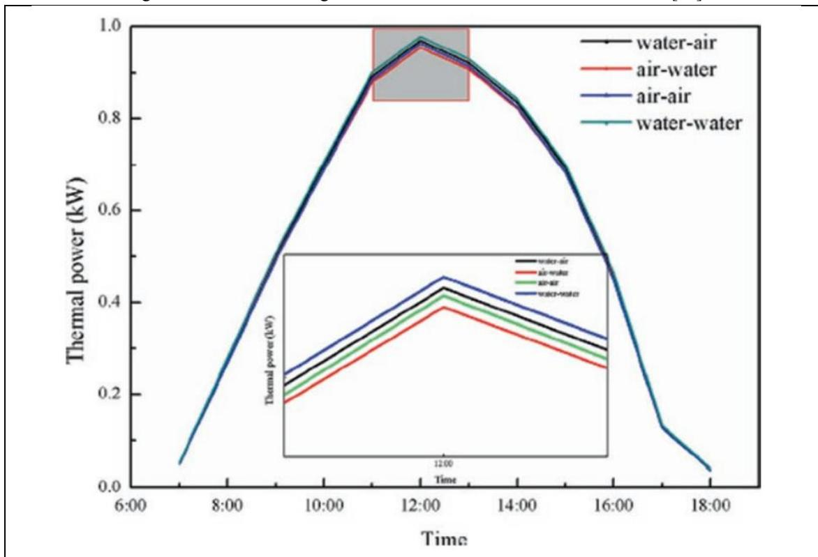
Fig. 11 The hourly variation of thermal power corresponding to different working fluid configurations [49]
