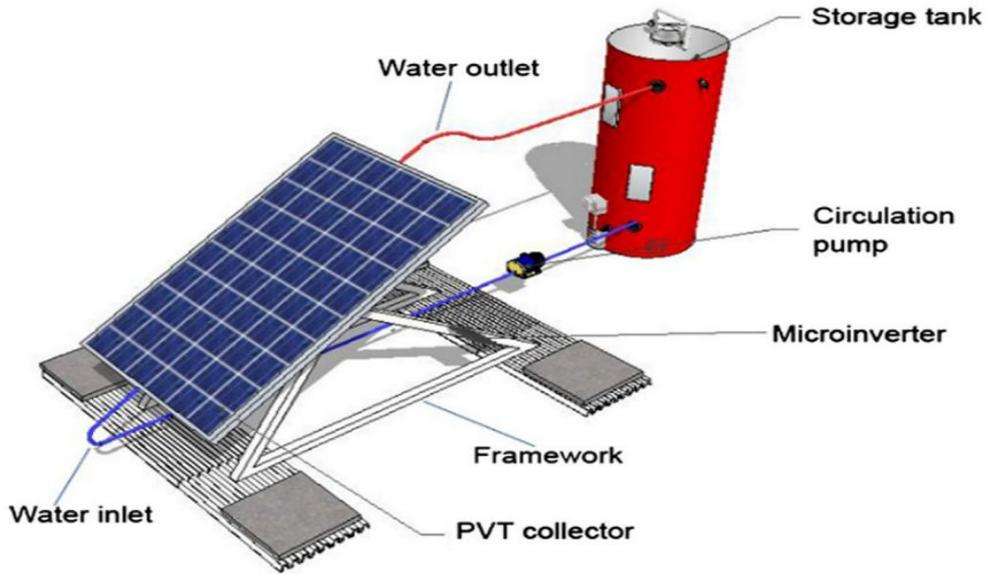
Figure 2: Uncovered PV/T collector configuration (Aste et al. 2016).
