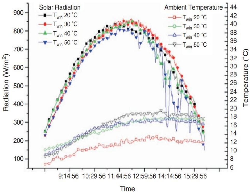
Fig. 6 Daily variation of solar irradiance (referred to as solar radiation) and ambient temperature during the experiment period [53]
