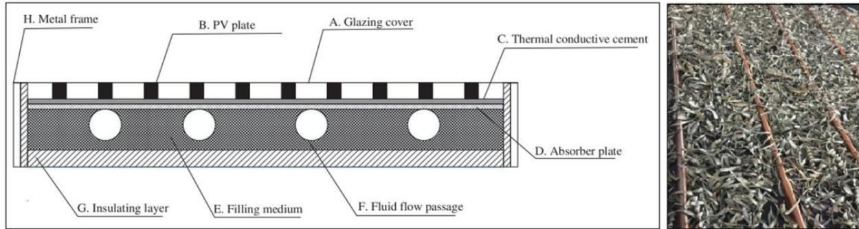
Figure 4: Cross section of the PV/T system and iron scrap filling (Ma et al. 2020).
