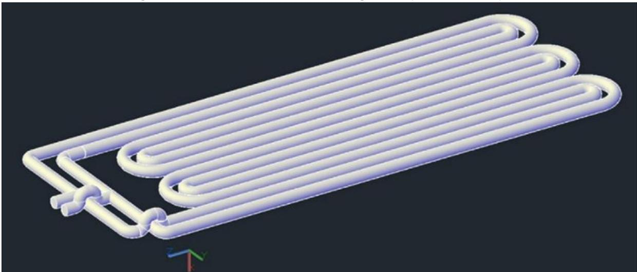
Figure 3: Dual oscillating absorber designed by Misha et al. (2019).
