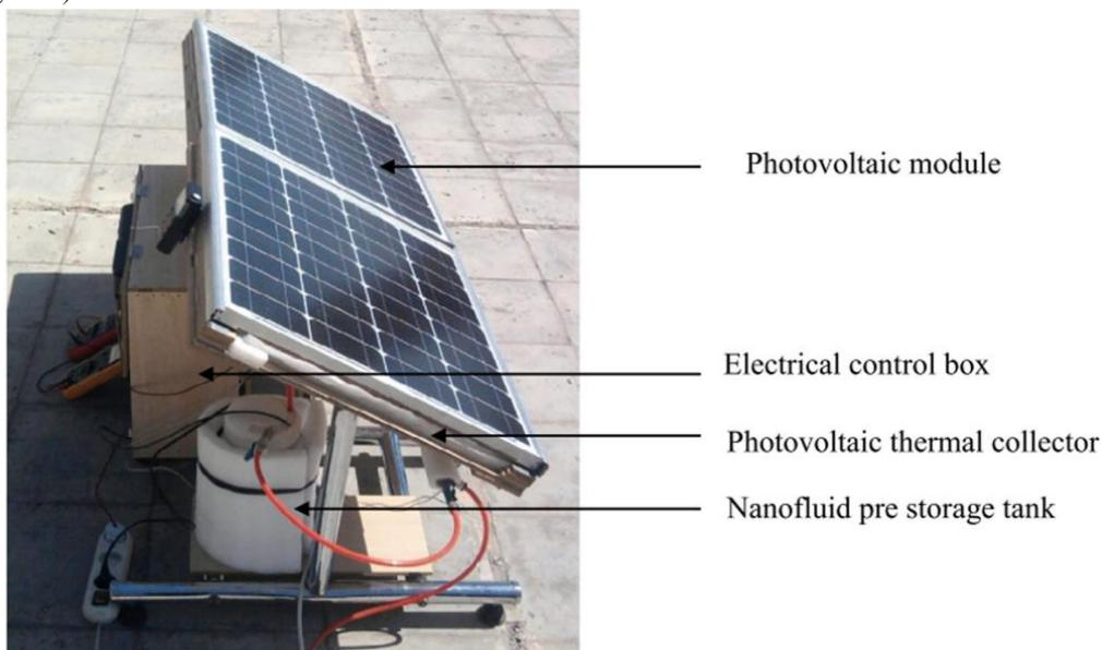
Figure 7: Experimental setup of the PV/T system studied by Rejeb et al. (2016).
