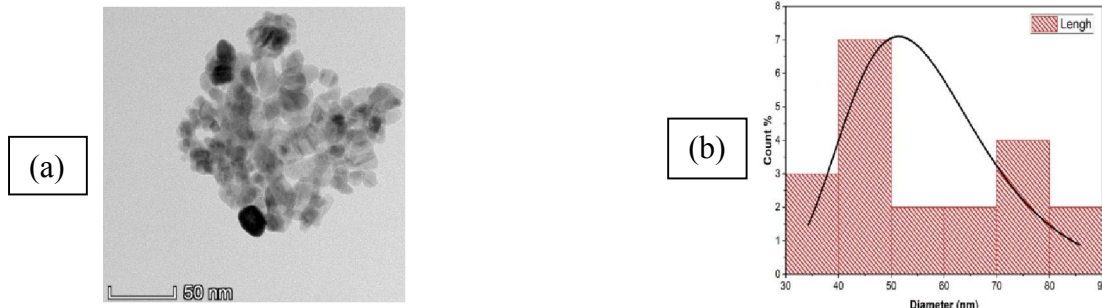
Fig 7. a) HR-TEM image b) Histogram of APT copper oxide nanoparticles
