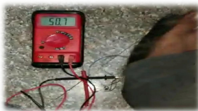
Figure 11. Voltage obtained through piezoelectric device
