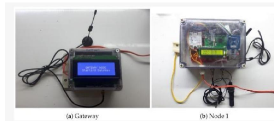
Figure 6: The prototype of the two boxes: gateway on the left and circuitry with all sensors of Node 1 on the right.
