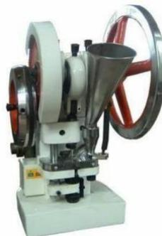
A tablet press can be used to create tablets from pharmaceuticals, nutraceuticals, cleaning products, industrial pellets, and cosmetic products. Granulated powder material is metered into a cavity made by two punches and a die, and then the material is fused together by applying high power to the punches, which is how tablets are made.[17]
