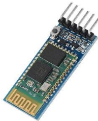
Figure 2: HC-05 bluetooth module
