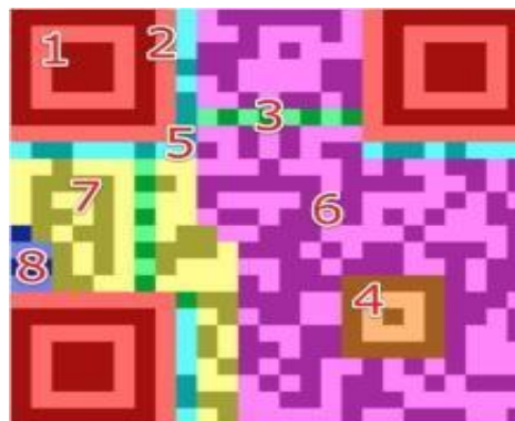
Figure 2. Structure of QR Code [3]
