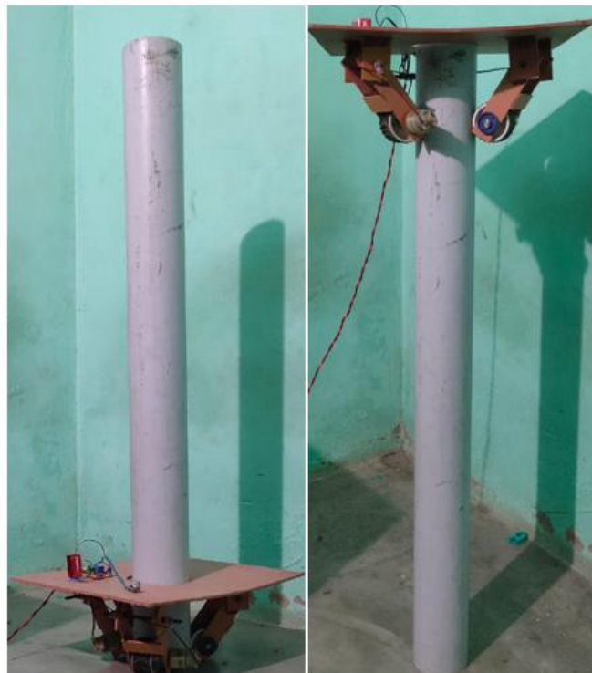
Fig. 6.1 Top and bottom position of PVC pipe climbing device
