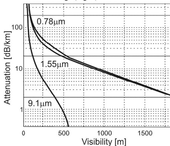
Figure 6. Dependence of visibility on attenuation coefficient for three spectral ranges: NIR, SWIR, and LWIR.
