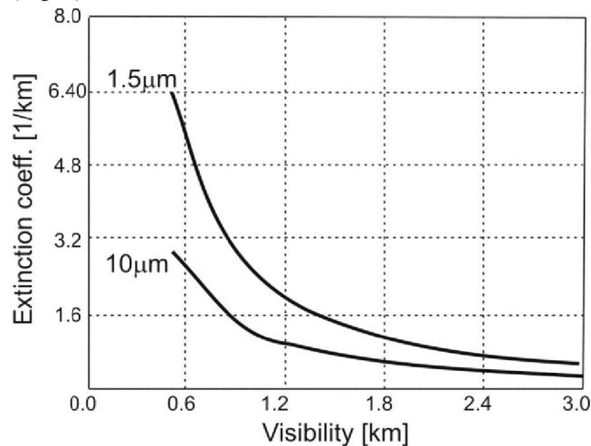
Figure 5. Extinction coefficient vs. visibility for two wavelengths: 10µm and 1.5µm.
