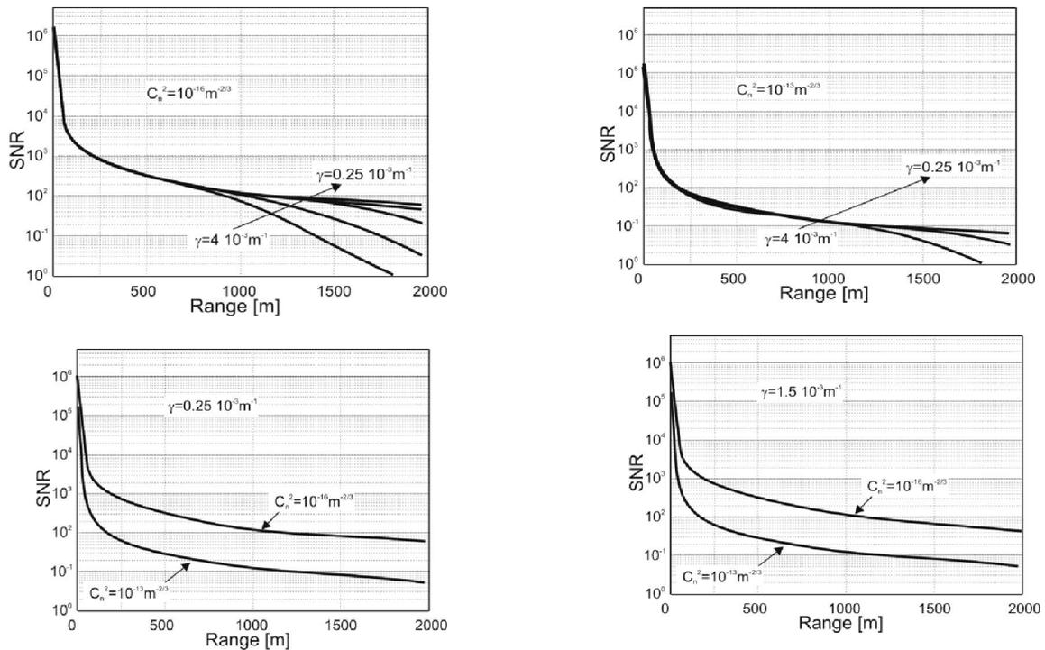
Figure 8. SNR dependence on the data link range of the developed FSO prototype for various weather conditions (determined by  $\gamma = 0.25m^{-1}$  - visibility better than 10 km, and by  $\gamma = 4m^{-1}$ , visibility of 0.5 km)
