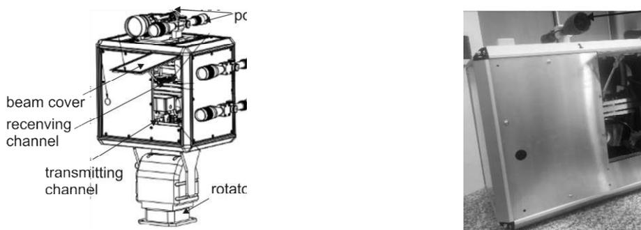
Figure 3. 3D model and view of the FSO head (transceiver and receiver).
