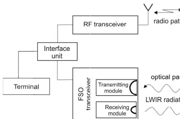
Figure 2. Block diagram of the FSO/RF hybrid link prototype.
