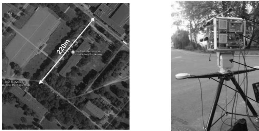
Figure 4. View of the test conditions and the FSO transceiver with GPS positioning system.
