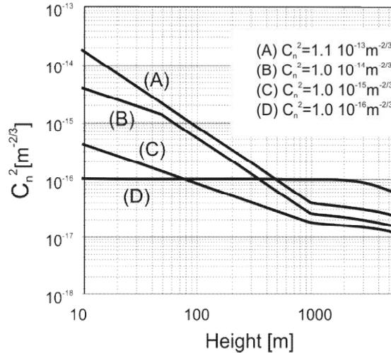
Figure 7.  $C_n^2$  parameter vs. height determined for the Gurvich model with four turbulence levels [10]
