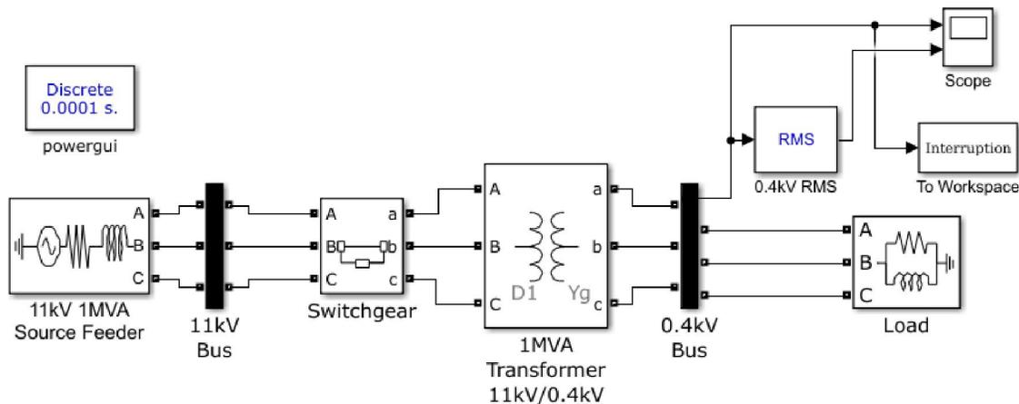
Fig. 3 MATLAB Simulink Model for Voltage Interruption
