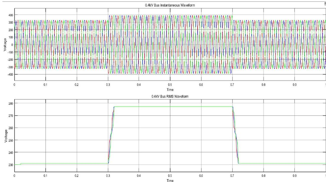
**Fig. 10** Voltage Waveform with 20% Swell
