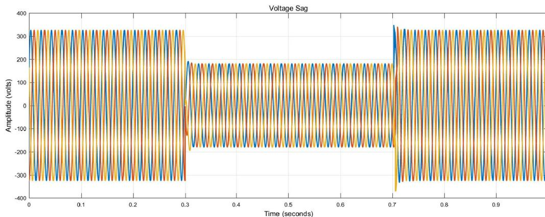
**Fig. 12** Voltage Waveform with 50 % Sag
