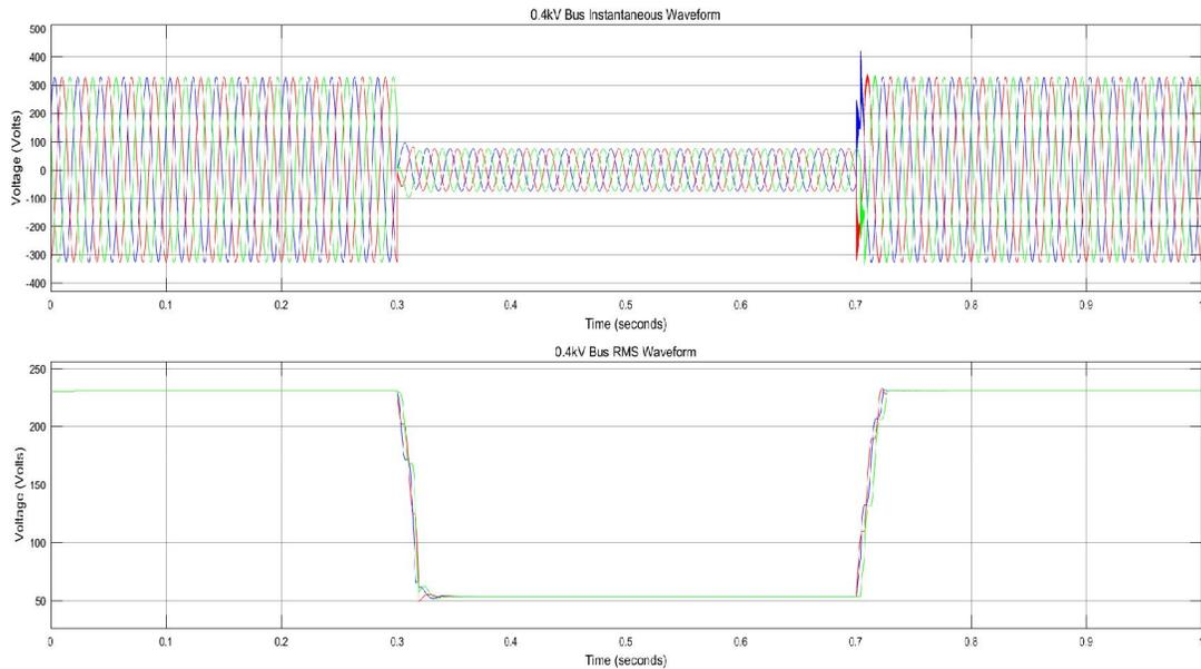
**Fig. 9** Voltage Waveform with 80 % Sag
