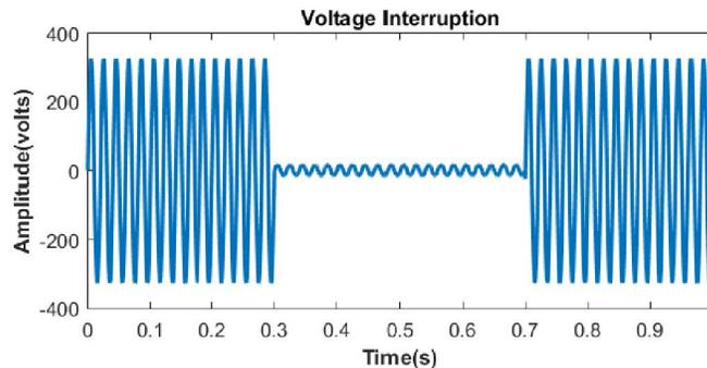
**Fig. 8** Voltage Waveform with Interruption
