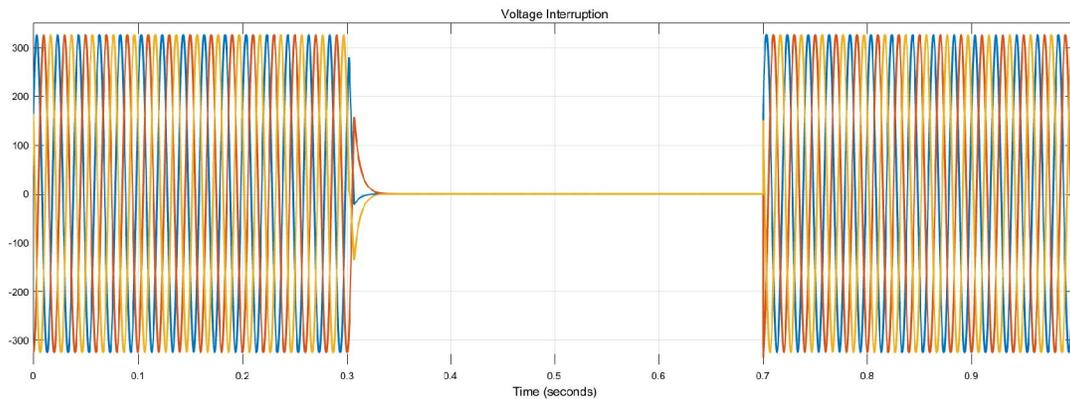
Fig. 14 Voltage Waveform with Interruption
