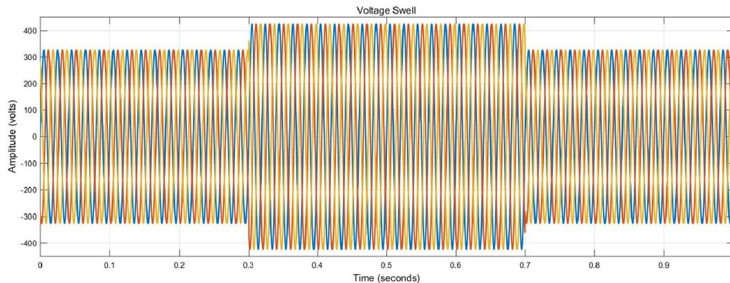
Fig. 13 Voltage Waveform with 20% Swell
