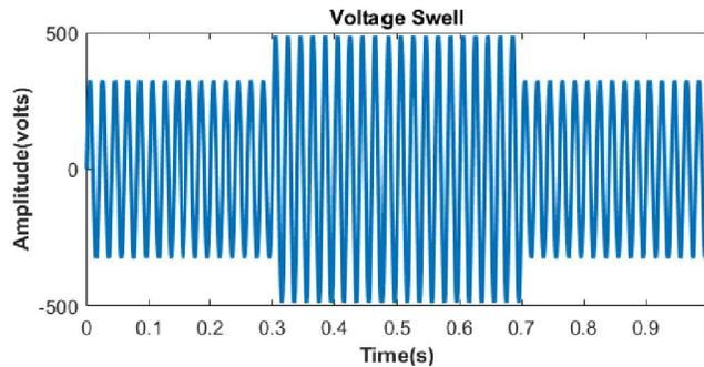
**Fig. 7** Voltage Waveform with Swell
