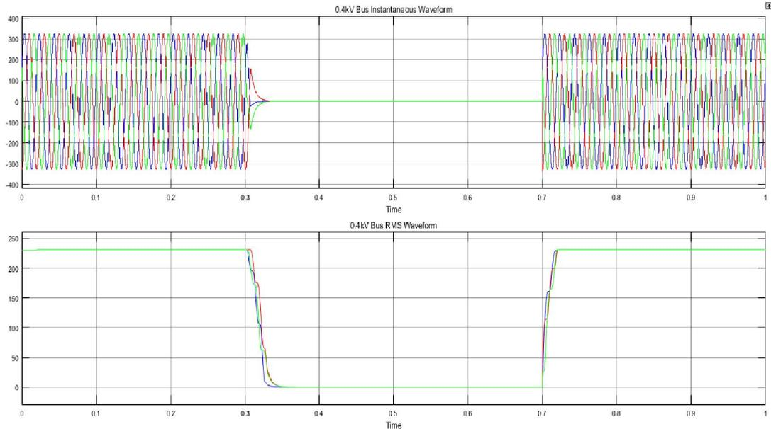
**Fig. 11** Voltage Waveform with Interruption
