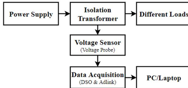
Fig. 5 Block diagram of Data Acquisition System
