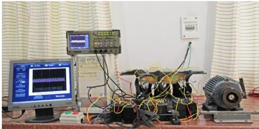
Fig. 4 Experimental setup for generation of PQDs
