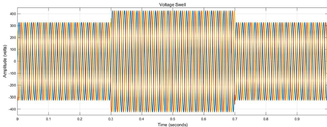
Fig. 13 Voltage Waveform with 20% Swell
