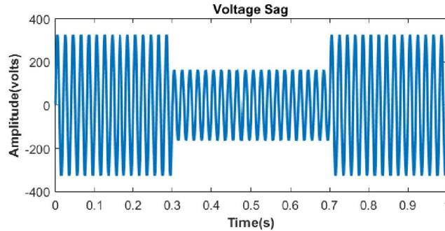
**Fig. 6** Voltage Waveform with Sag
