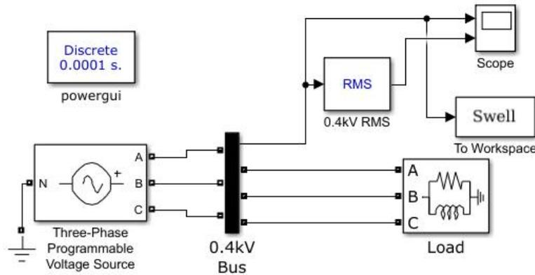
Fig. 2 MATLAB Simulink Model for Voltage Swell
