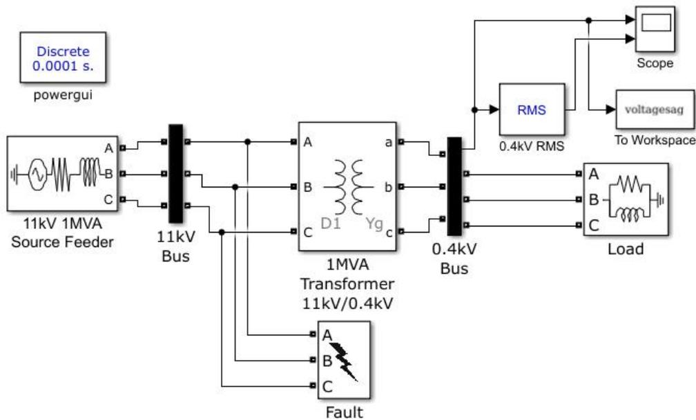
Fig. 1 MATLAB Simulink Model for Voltage Sag
