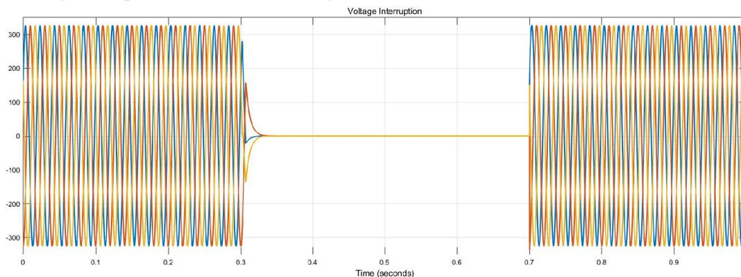
Fig. 14 Voltage Waveform with Interruption
