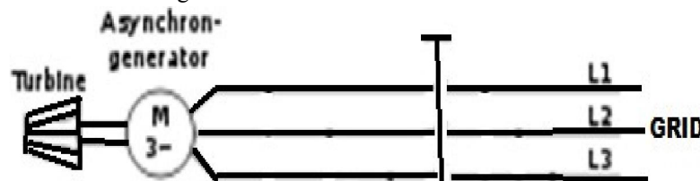
Figure 1 Schematic diagram of a grid-excited induction generator.
