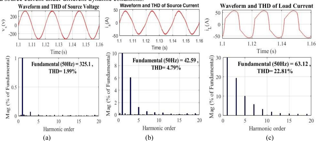
Fig. 7(a)-(c) Harmonic analysis of source voltage, source current and load current
