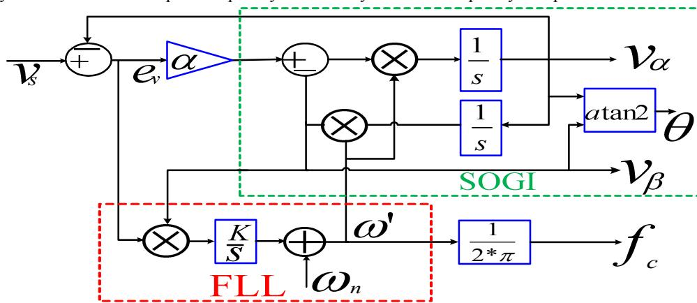
Fig. 2 Structure of SOGI-FLL for synchronization
