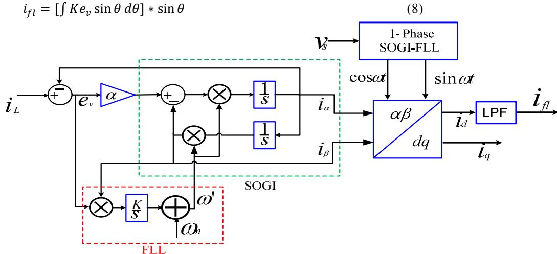
Fig. 3 SOGI-FLL control algorithm
