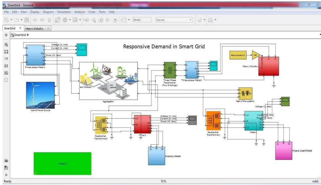
Fig 1 Simulink model for Demand Response Management
