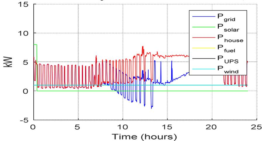
Fig 2 Demand (KW) P<sub>house</sub> from houses and Grid Response for various sources Solar, House, fuel and Wind sources.
