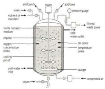
Batch bioreactors consist of a single tank capable of carrying out sequences of reactions and are easy to operate. The tank is equipped with an agitator (stirred tank reactor – STR) to mix the reactants along with an integral heating and cooling system. Buffer solution or pH controller is used to control pH of the reactant. These vessels may vary in capacity
