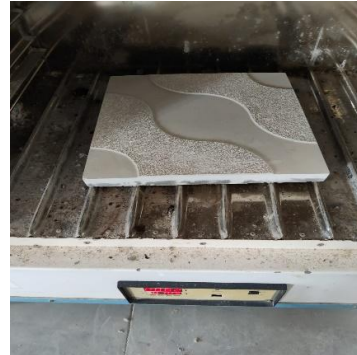
Fig. Tiles in oven for drying
