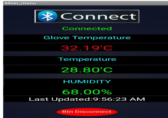
Fig. 4. Temperature readings following Bluetooth connection
