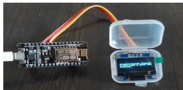
Figure 3: Inter Facing of OLED and ESP8266
