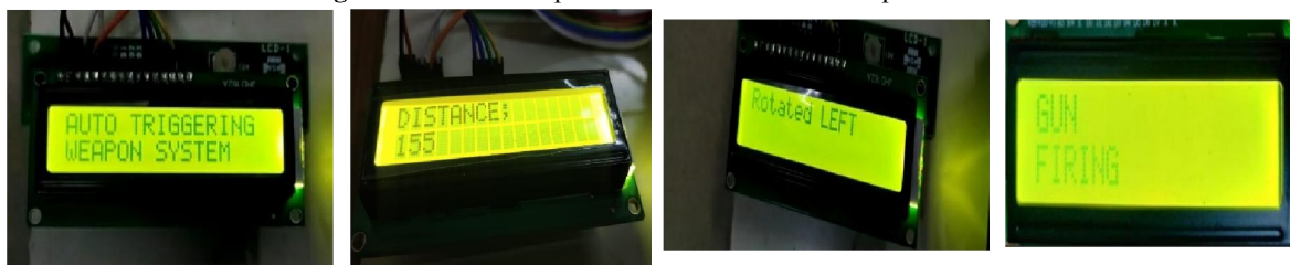
Fig 5: LCD Display showing (a) Name of our project (b) Distance of the intruder (c) Weapon arm direction (d) Triggering status
