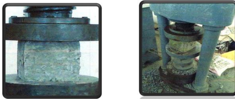
Fig 1.6 Testing of Cubes
