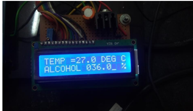
Fig. Temperature and Alcohol Sensor output observed on the LCD
