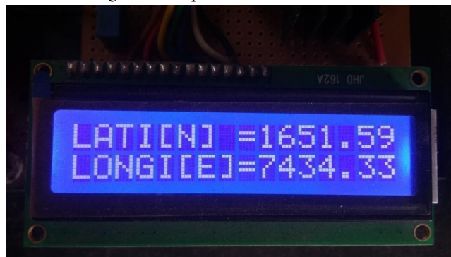
Fig. GPS output observed on the LCD
