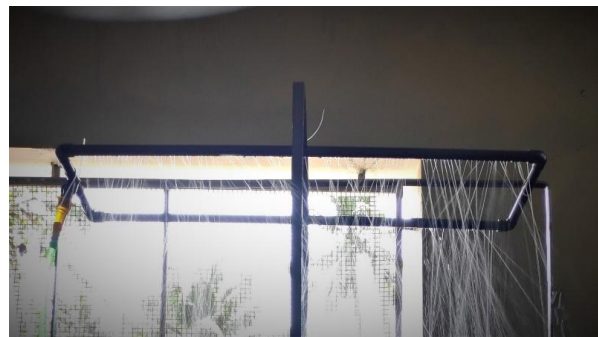
Fig 6: Artificial rainfall system
