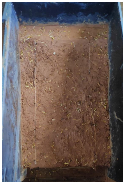
Fig 12: Composite reinforced slope before simulated rainfall
