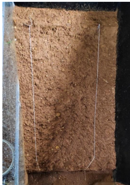
Fig 11: Geocell supported slope after simulated rainfall
