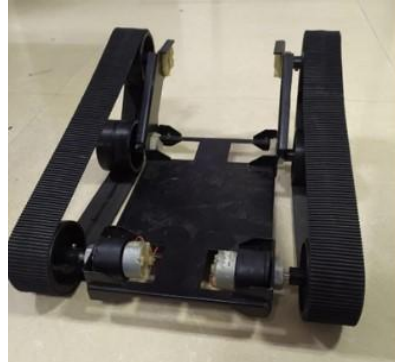
Fig. 2. Mechanical base of the robot with motors
