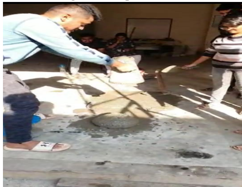
Fig 6.3 Slump Cone Test
