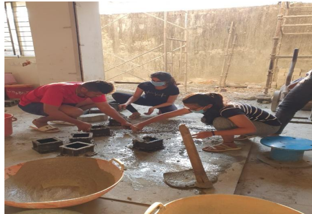
Fig 6.4 Casting of Mould
