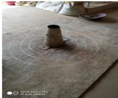
Fig 6.2 Slump Cone Test
