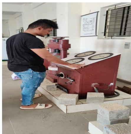
Fig 8.1 Compressive strength Test Conduction
