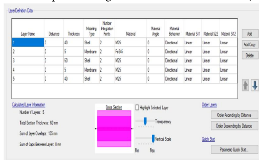
Fig 6.7 Floor Slab Properties
