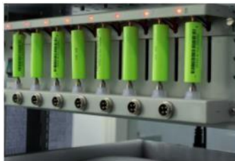
Cell Capacity Grading
