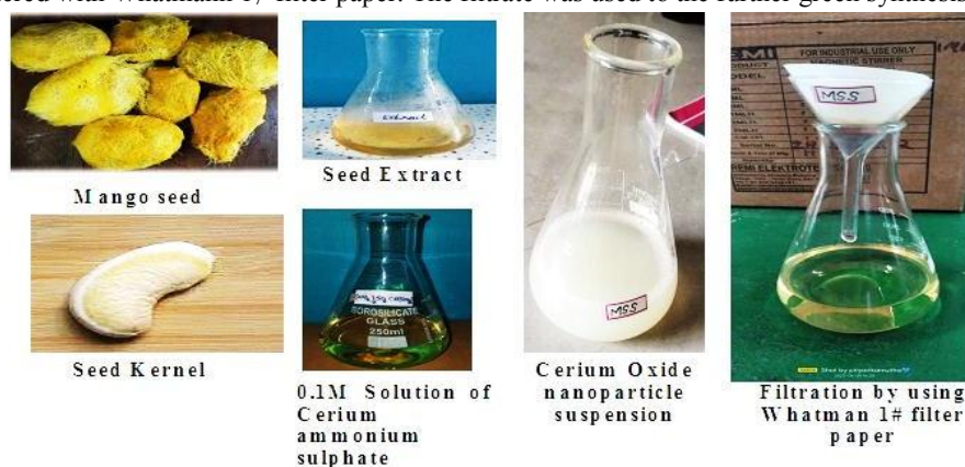
Figure 1: Green synthesis of Cerium oxide nanoparticles mediated by Mango seed kernel extract
