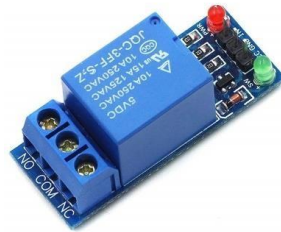
Figure 5: 5v DC Relay Switch
