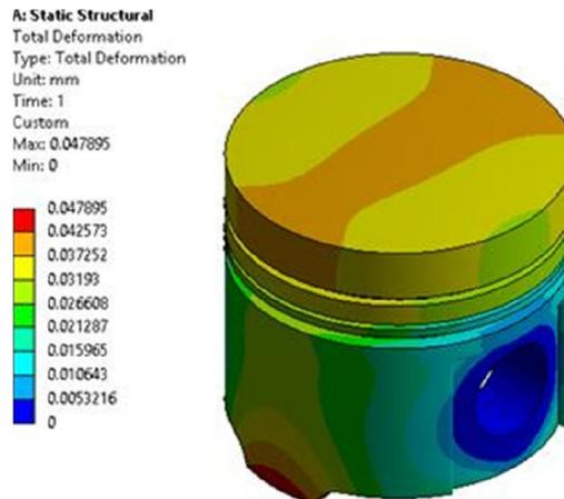
**Figure 7:** Total Deformation on piston
