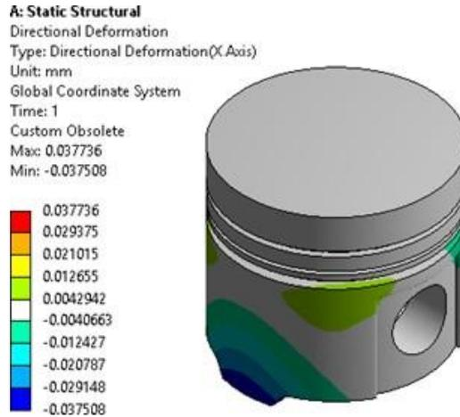
**Figure 14:** Directional Deformation on honeycomb structured piston
