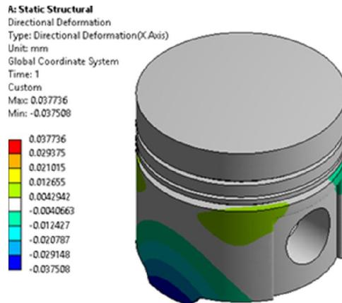
**Figure 8:** Directional Deformation on piston
