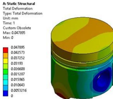
Figure 13: Total Deformation on honeycomb structured piston
