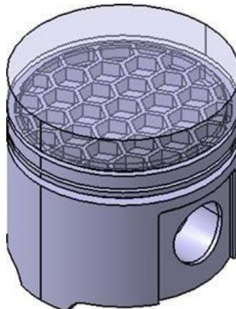
Figure 2: Honeycomb Piston
