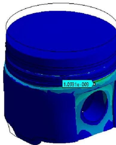
**Figure 16:** Equivalent Elastic Strain
