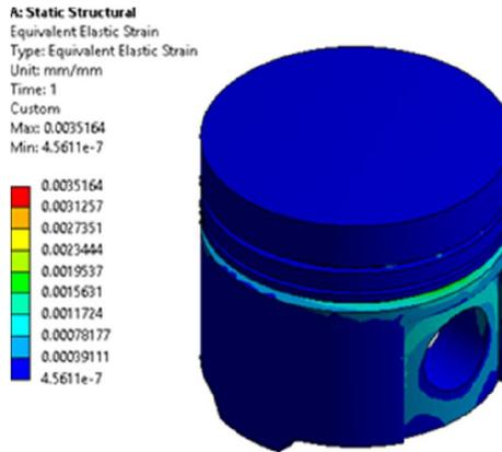
**Figure 6:** Equivalent strain on the piston
