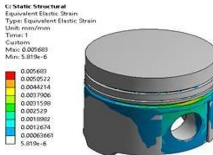
Figure 12: Equivalent strain on honeycomb structured piston
