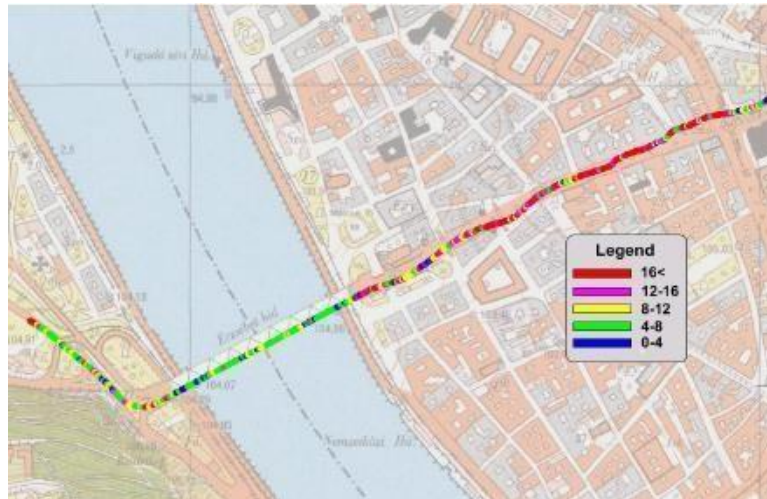
Figure 7: IRI map derived from laser markers below the tires [23]
