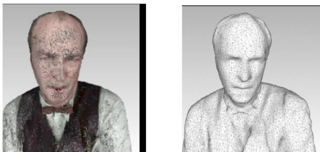
Fig 5: Example for a resulting depth map by one of the 16 stereo systems (top) and close-up of fused point cloud with 20M 3D points (middle) and simplified mesh with 70k faces (bottom)
