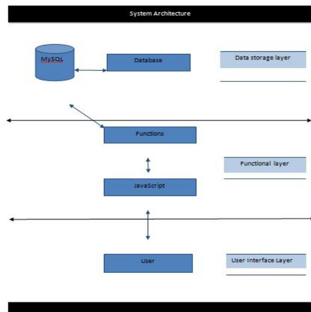
Fig. 1. Architecture Diagram
