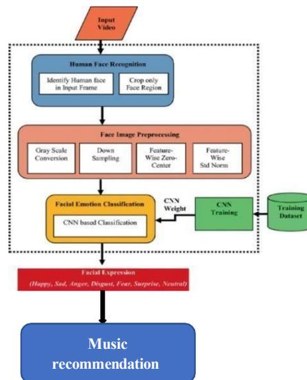
Fig. 2. System Architecture
