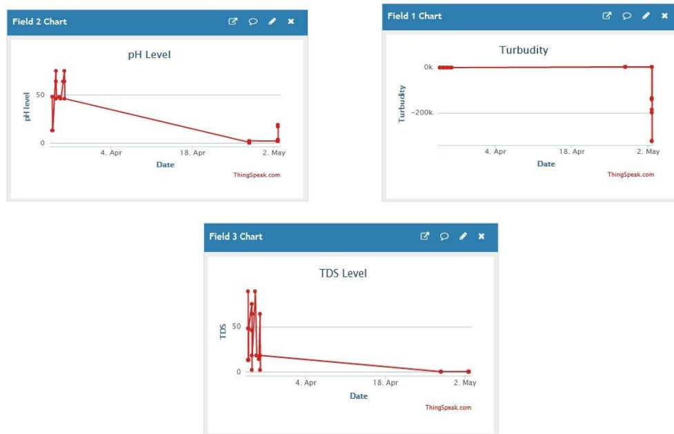
Fig shows that location-1-water source sensors information displayed on the Thing speak .This information can be accessed from anytime and anywhere and the concern person take the decision accordingly.
