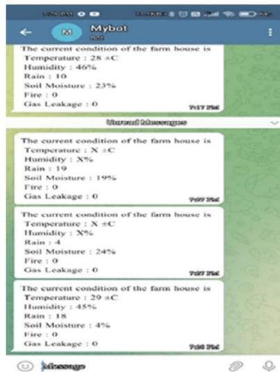
Fig 12. Data received on Telegram
