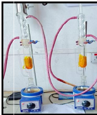
Fig. 2: Extraction of curcumin by soxhlet
